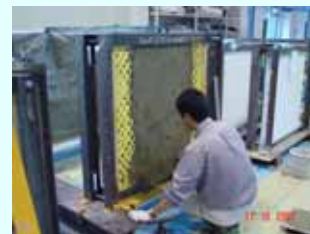
7. Mortar laying (cement mortar in this case)
