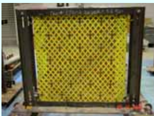
5. Masonry wall with mesh before mortar laying
