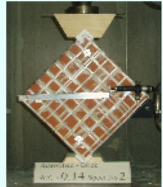
Specimens were tested 28 days after construction under displacement control condition. The loading rate was 0.3mm/min and 2mm/min for the non-retrofitted and retrofitted cases, respectively.
