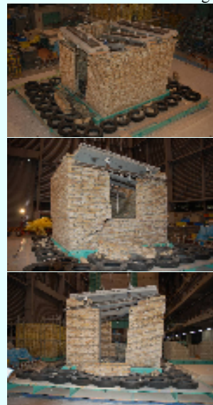
Input motion: Sinusoidal wave, f=3\text{ Hz} , Amp=600 Gal, 60s
