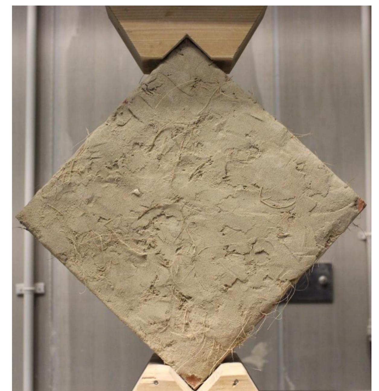
Fig. 3. Diagonal compression test of fiber reinforced cement composite
