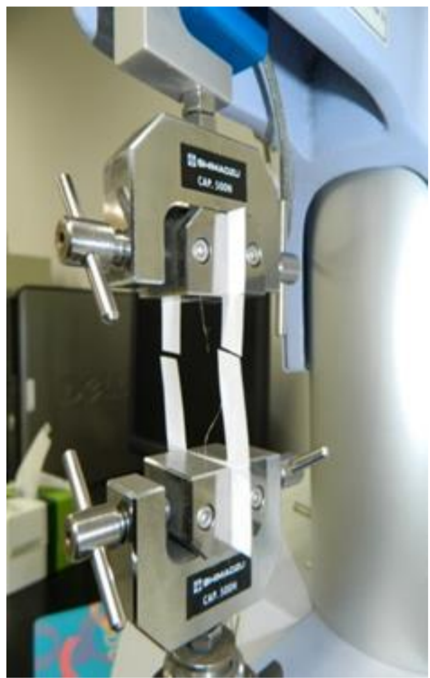
Fig. 1. Tensile test of abaca fiber
